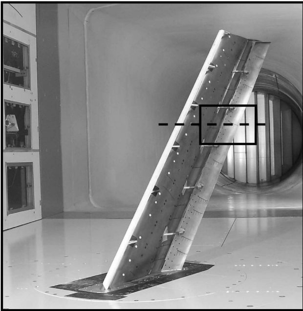
Fig. 3 AFV wing mounted in ONERA's F1 wind tunnel, showing the spanwise actuated flap section and the location of pressure measurement tapings.
